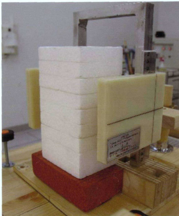
Fig.22 Brain biopsy phantom attached to the device.
