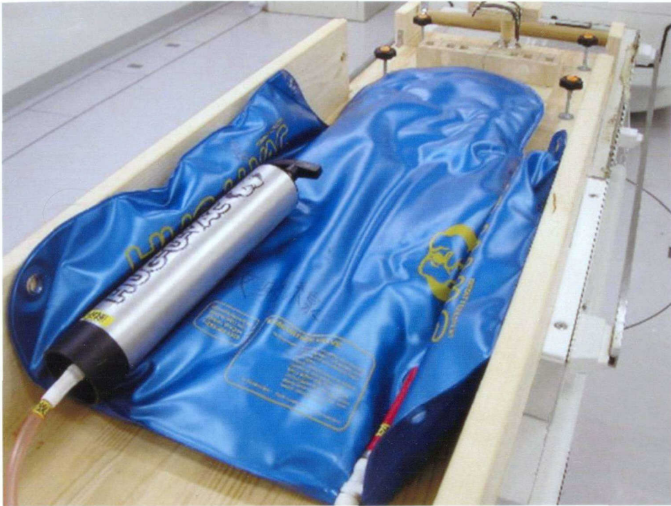
Fig.17 An inflatable pillow (HUG-U VAC: sports doc Inc.) used to support the neck and body. The air in the pillow was evacuated so the pillow conforms to the shape of the dog.
