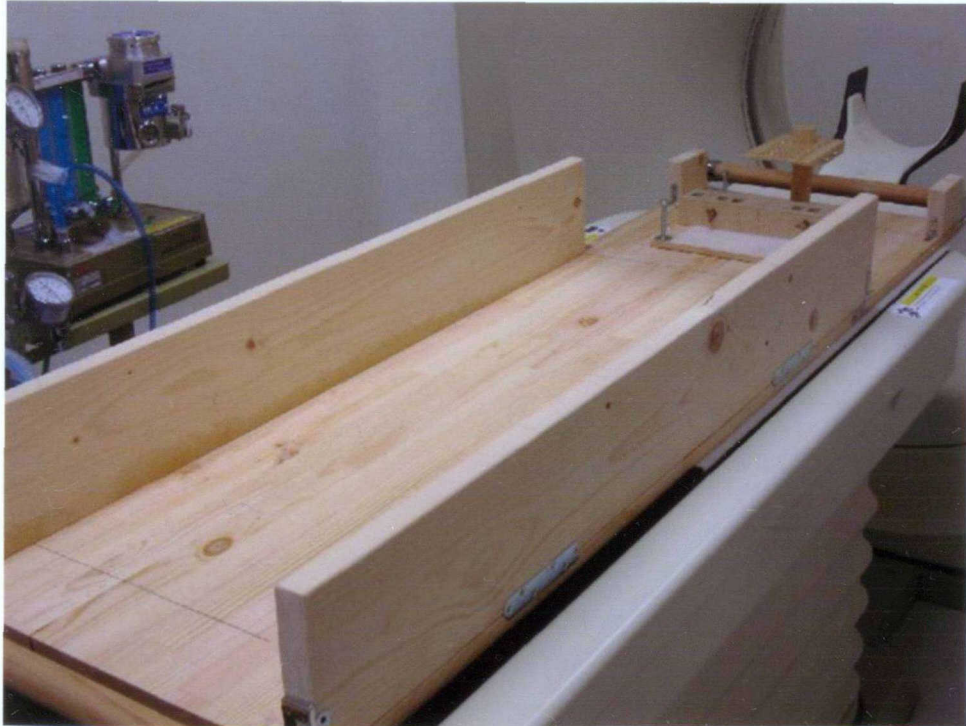
Fig.14 A test model of the stereotactic brain biopsy device for small animal.
