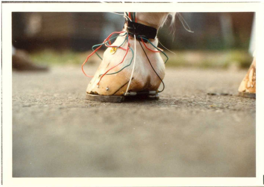
Fig. 7 Photograph showing the fore hoof with strain gauges and transducer.
